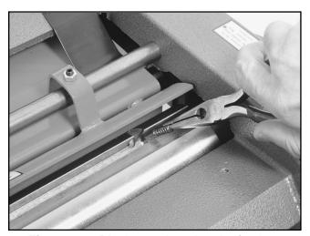
Figure 14. Placing springs into knife slots.
